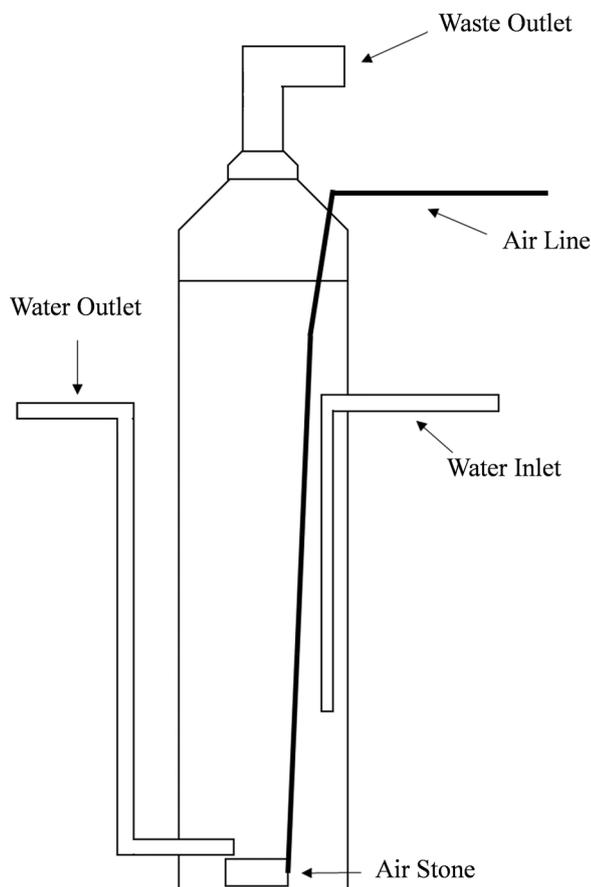
Fig. 1. The design of the PVC foam fractionators used for this project.
